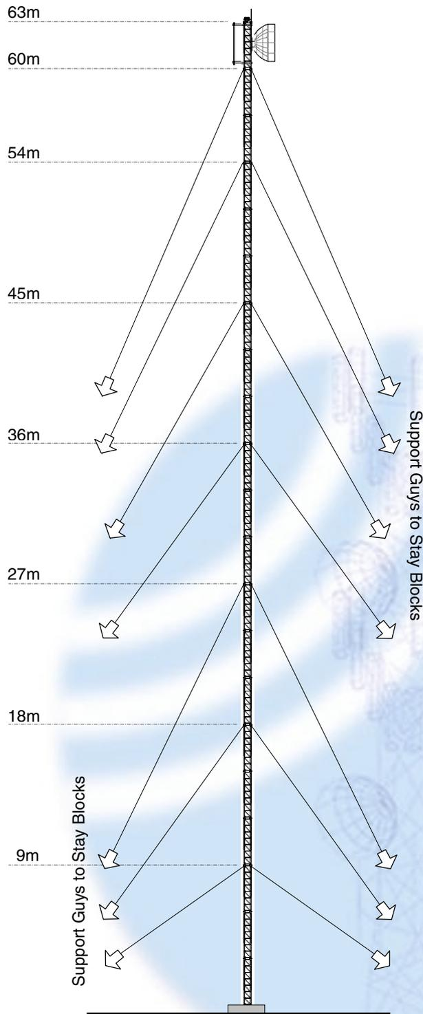
**GM - 440: A medium duty mast for grid antenna and medium-wave applications**
